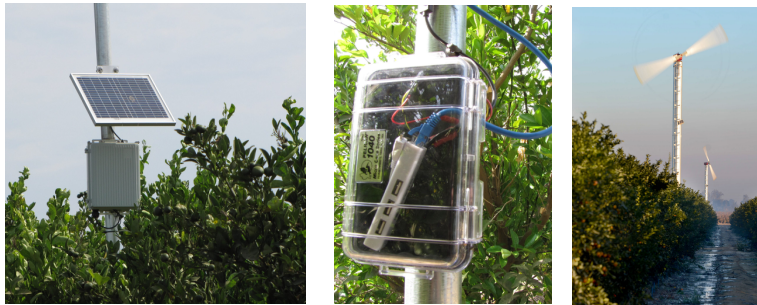
Solar panels and sensors will help researchers know when to turn on windfans to protect citrus trees from frost.
