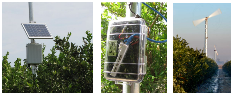
Low-power and low-cost IoT deployment such as solar panels and sensors will help researchers know when to turn on windfans to protect citrus from frost.
